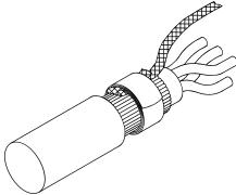
3. Wind the remainder of the constant force spring onto the cable assembly.
