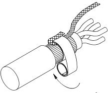
2. Apply 2-3 turns of the constant force spring, then turn the earth braid/cable back on the spring.
