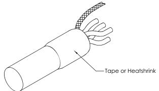
4. Apply tape or heat shrink to cover the spring and armour/screen, spring and earth braid/cable assembly.
