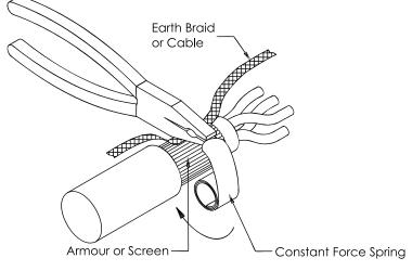
1. Strip cable sheath off the metallic armour or screen and lay the braid or earth cable on it lengthways. Start winding the constant force spring over both armour/screen and earth braid/cable
